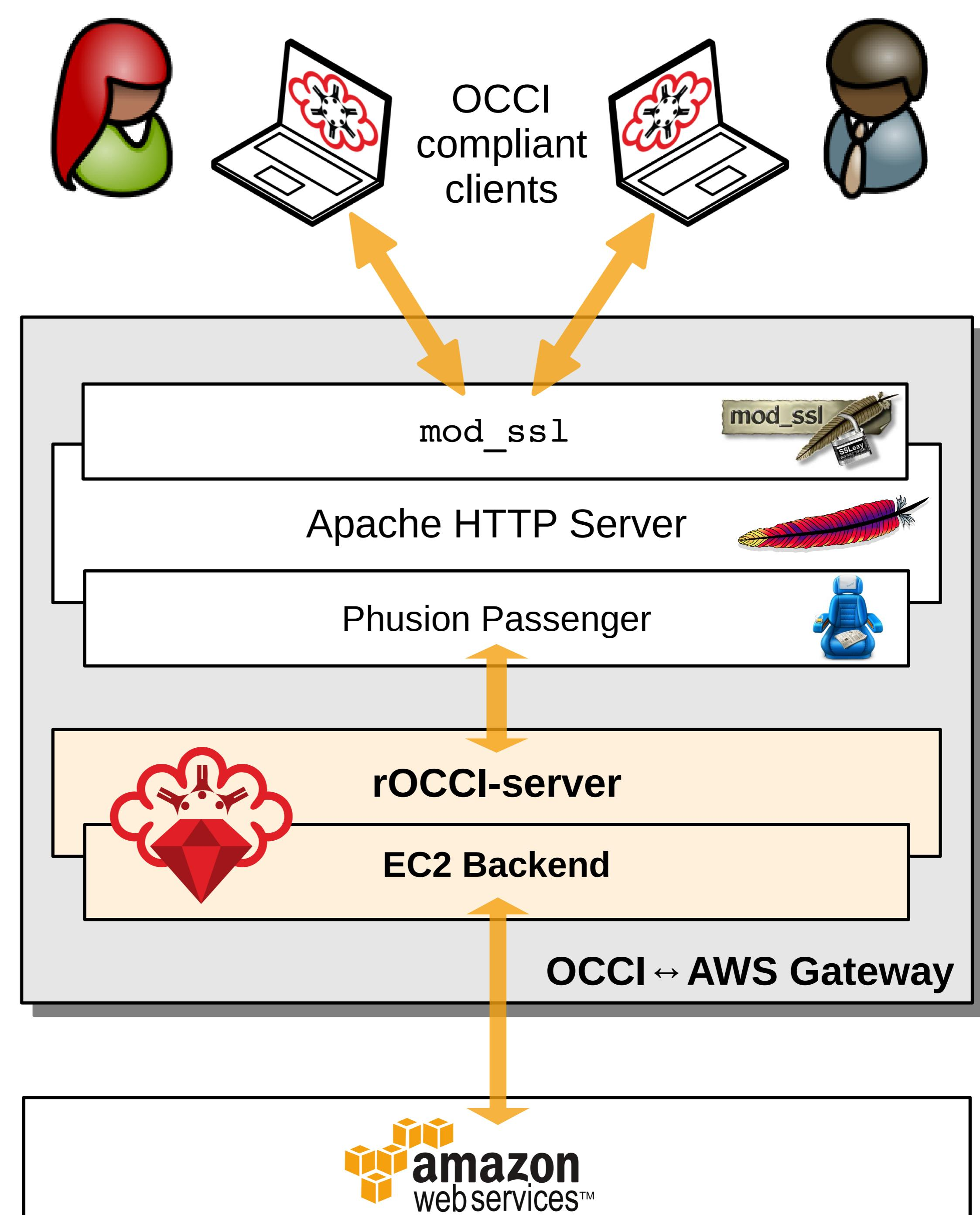
For use with AWS EC2, the rOCCI-server is simply configured to use its EC2 backend, which is part of the standard release.
