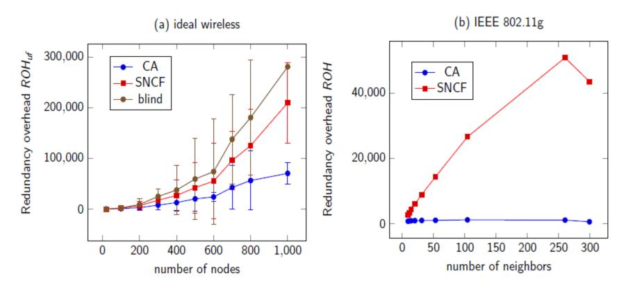
SNCF - simple flooding, CA - proposed cellular automate based protocol
