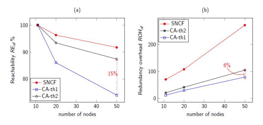
Threshold can be tuned to tradeoff between reachability and redundancy
