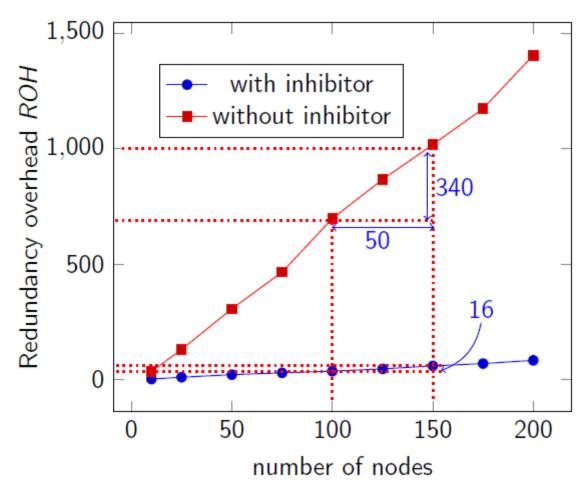
Rate of growth with inhibitor < that without inhibitor
