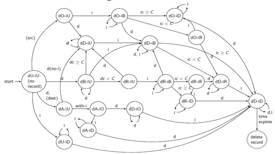
d-data, i-inhibitor, U-unknown, O-originated, B-buffered, R-rebroadcast, D-discarded, A-accepted, c-concentration, C-threshold
