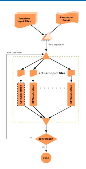
This workflow shows how a differential evolution optimizer is implemented with the GC3Pie library to support the analysis of a computationally intense economic model.
